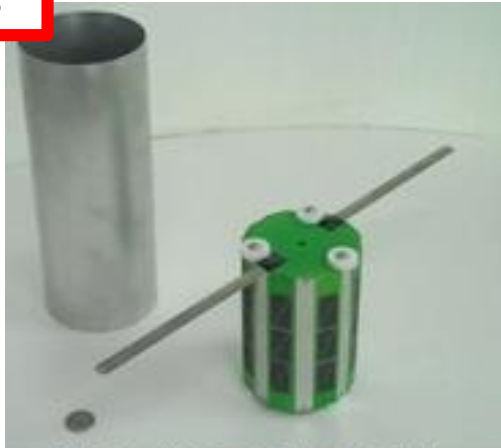
TubeSat with Sample Ejection Cylinder
